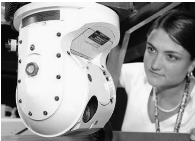
FIGURE 12.11 Turret of built-in BAE Jeteye countermeasure system.
