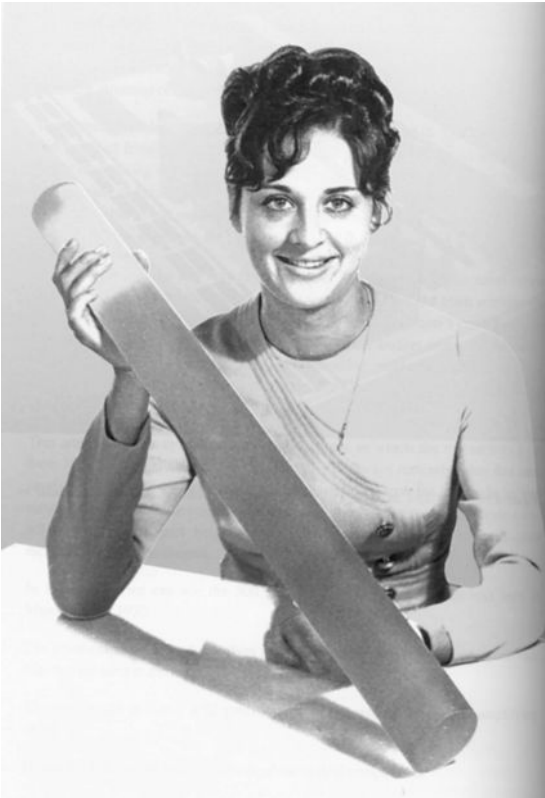
FIGURE 13.2 Nd:glass rod in 1970 French inertial confinement laser and amplifier.
